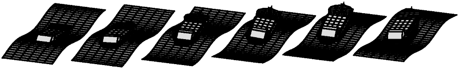
Figure 13. Ship C in following seas, with wave heights of H = 9.8 \text{ m} . The rudder is fixed but the ship is free to yaw, so that the heading angle varies around \mu = 0^\circ .
